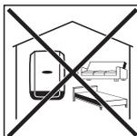
As the inverter generates low levels of noise at certain times, it should not be installed close to living areas.
