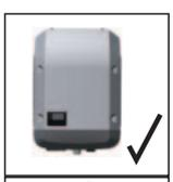
The inverter is designed to be installed vertically on a vertical wall or pillar.
