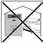
As the battery generates low levels of noise under certain operating conditions, it should not be installed close to living areas.
