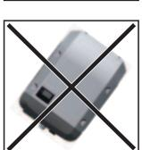
Do not install the inverter at an angle on a vertical wall or pillar.
