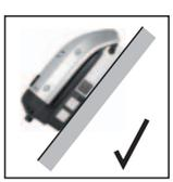
The inverter is suitable for installation on a sloping surface.
