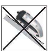
Do not install the inverter on a sloping surface with its connection sockets facing upwards.
