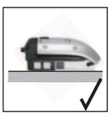
The inverter is suitable for horizontal installation.
