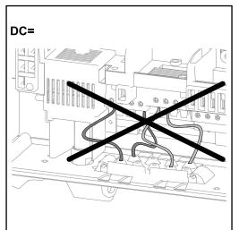
If DC cables are laid over the shaft of the DC main switch or across the connection block of the DC main switch, they may be damaged when the inverter is swung in, or they may even prevent the inverter from being swung in.
