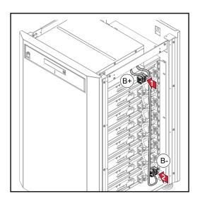
Check the voltage between  $U_{B_-}$  and  $U_{B+}$
