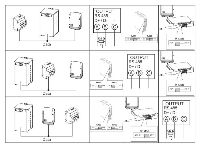
\*) The R 120 Ohm terminating resistor is included with the Fronius Smart Meter
