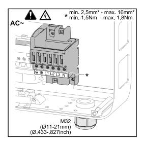
PE Ground conductor / grounding
