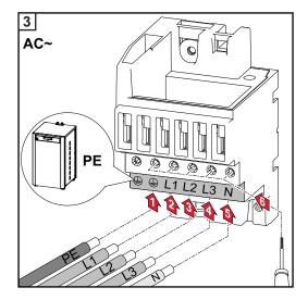
If AC cables are laid over the shaft of the DC main switch or across the connection block of the DC main switch, they may be damaged when the inverter is swung in, or they may even prevent the inverter from being swung in.
