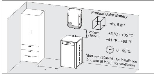
\* a lateral clearance of 500 mm is required when installing the battery modules in the battery cabinet
