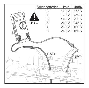
**IMPORTANT!** Check the voltage of the battery modules.
