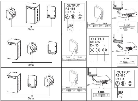
\* The terminating resistor is included with the Fronius Smart Meter
