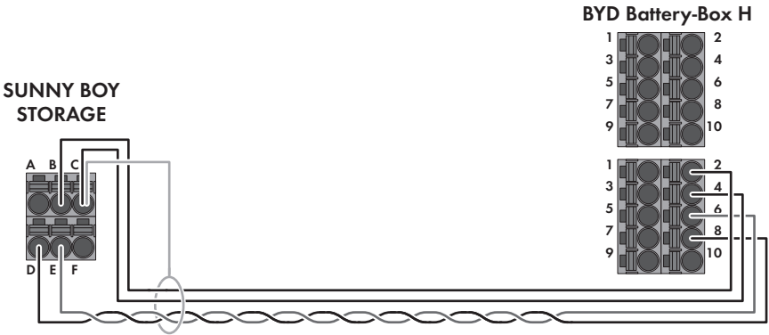
Figure 2: Cabling plan SBS2.5-1VL-10 with Battery-Box H
