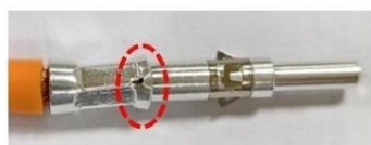
The length of the copper wire inserted into the terminal is too short, and the copper wire is not visible in the observation hole.
