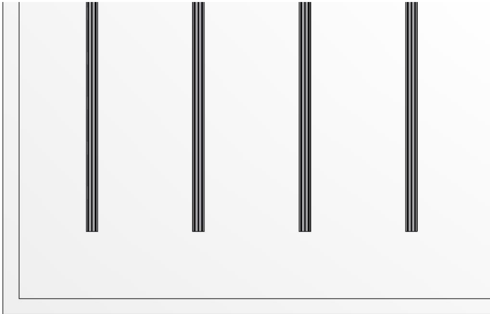
Fig. 19 Align the base rails so that they are parallel and vertical.
